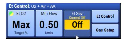
Figure 9: Selecting end-expired O<sub>2</sub> and agent target concentrations
