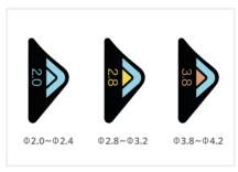
Labels attached to the control portion, which show the model number and instrument channel inlet size
