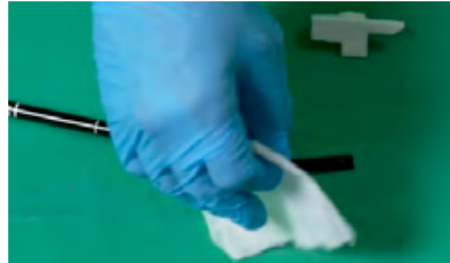
4. Sterilise the endoscope and the setting tool with alcohol.
