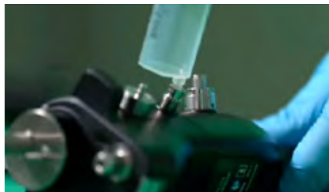
3. Insert endoscope into the overtube. Push air through the supply port with an empty syringe to expel excess water.
