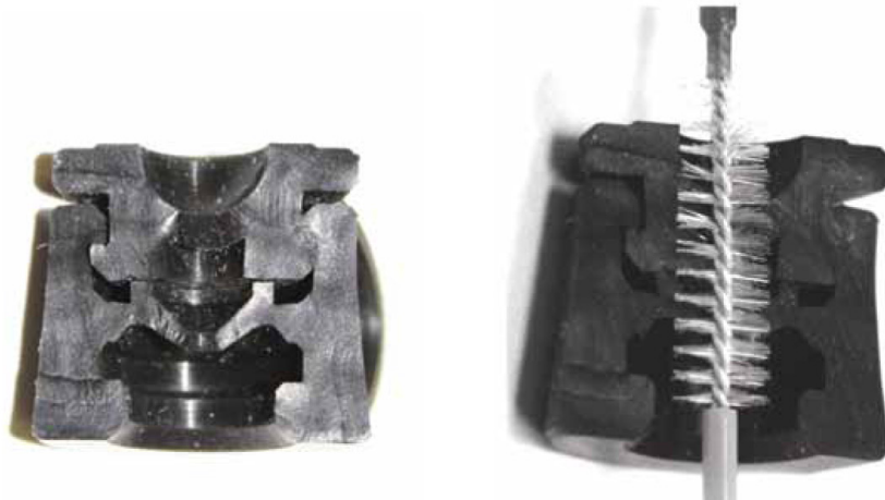
Exhibit B: Cross-sectional view of a typical reusable biopsy valve, demonstrating the nooks and crannies that make a reusable valve difficult to clean.
