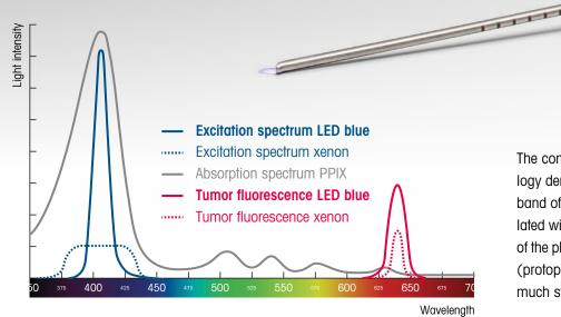
The comparison with xenon technology demonstrates that the emission band of **LED blue** is optimally correlated with the main absorption band of the photosensitizer based on PPIX (protoporphyrin IX). This leads to much stronger tumor fluorescence.
