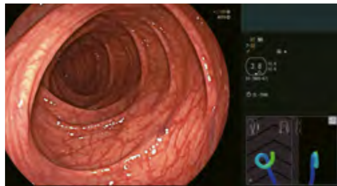
The endoscope shape is to be displayed on the monitor for VP-7000 by using the PoP function
